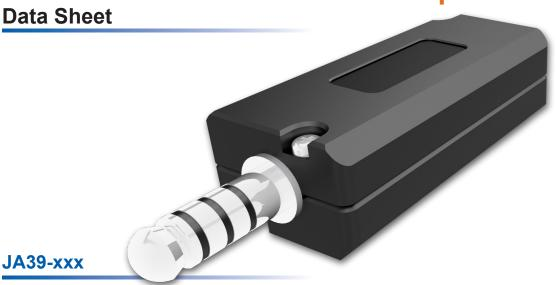
The JA39-xxx series of in-line headset adapters allow a variety of headset types and impedances to be used with a regular aviation audio controller such as the Jupiter Avionics JA95-xxx series. The adapter operates using the Mic. Bias supply of the audio controller and does not require any external power.
