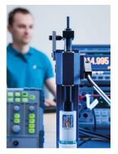
► Following the commands, each acoustic beacon is programmed and tested individually. Accuracy and calibration – a must to meet the requirements.
